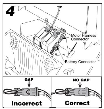
• Plug the battery connector and motor harness connectors together. Push firmly to make sure the two connectors are completely joined.
